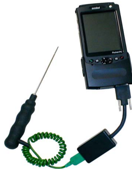
Versid KT-10s temperature acquisition module shown attached with a positive capture connector to the serial adapter attachment of the Symbol MC-50 mobile hand held computer. The industry standard thermocouple probe connector allows the use of your existing probes.
